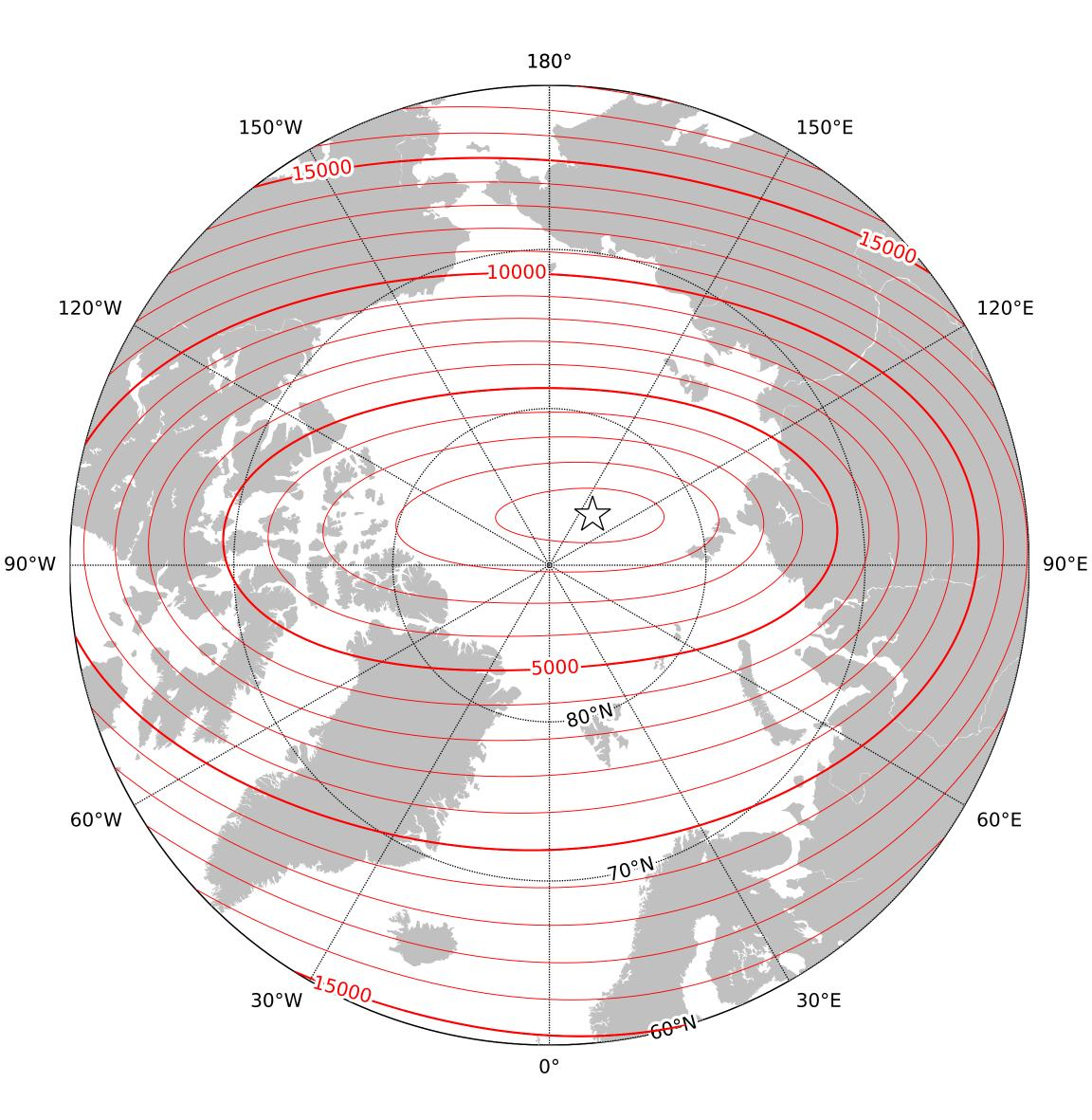
Horizontal Intensity (H) in the region of the north pole at 2025.0 from the World Magnetic Model (WMM) 2025. Contour interval is 1000nT, white star is the location of a magnetic pole and the projection is Polar Stereographic. This is an example of an isodynamic chart. British Geological Survey © UKRI 2024
