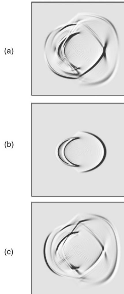
Figure 6. Snapshots of seismic wave fields for three components at time 0.28 sec in the two-layer transversely isotropic medium, computed by the NADM, for (a)  $u_x$  component, (b)  $u_y$  component, and (c)  $u_z$  component.
