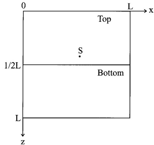
Figure 4. The model geometry.  $S$  denotes source.
