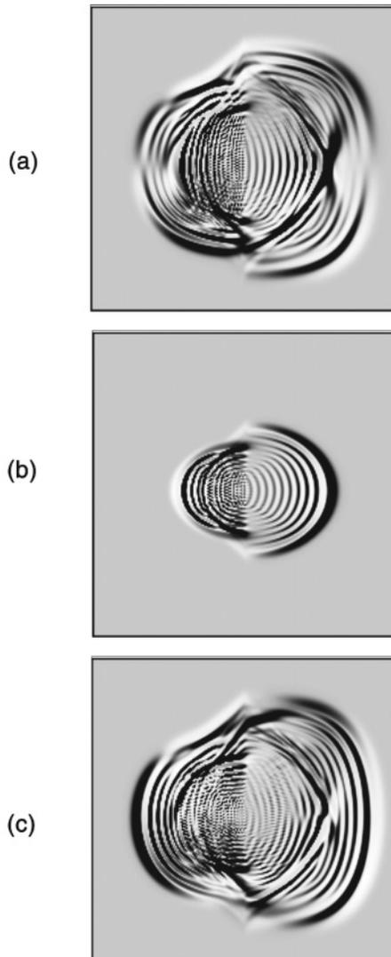
Figure 7. Snapshots of seismic wave fields for three components at time 0.28 sec in the two-layer transversely isotropic medium, computed by the conventional FDM, for (a)  $u_x$  component, (b)  $u_y$  component, and (c)  $u_z$  component.
