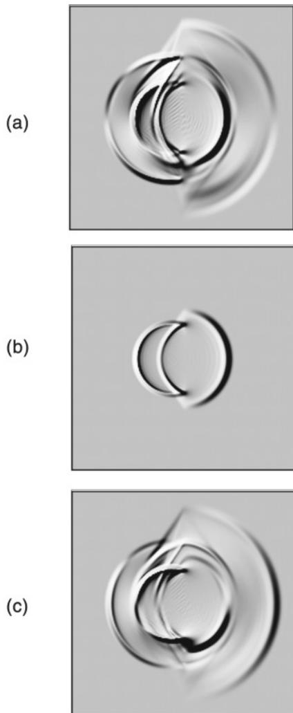
Figure 5. Snapshots of seismic wave fields for three components at time 0.56 sec in the two-layer isotropic medium, computed by the NADM, for (a)  $u_x$  component, (b)  $u_y$  component, and (c)  $u_z$  component.
