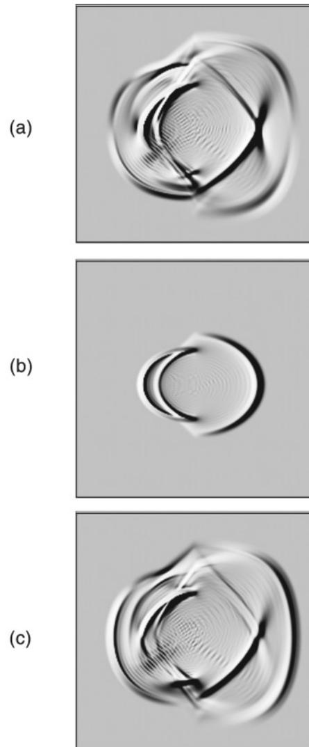
Figure 8. Wave-field snapshots for the coarse grid ( $\Delta x = \Delta z = 50$  m) at time 1.4 sec in the two-layer transversely isotropic medium, computed by the NADM, for (a)  $u_x$  component, (b)  $u_y$  component, and (c)  $u_z$  component.
