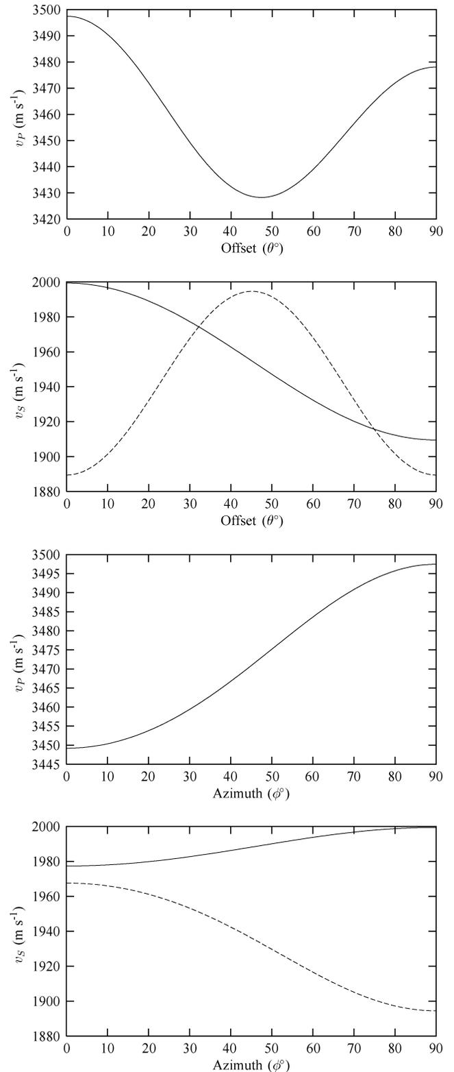
**Figure 1.** (a) The variation in compressional wave speed with offset at an azimuth parallel to the smallest crack dimension. (b) As in (a), but for shear wave speeds. The solid line corresponds to the quasi-SV wave and the dashed line to the quasi-SH wave. (c) The variation in compressional wave speed with azimuth at an offset of  $30^\circ$ . (d) As in (c), but for shear wave speeds. The solid line corresponds to the quasi-SV wave and the dashed line to the quasi-SH wave.
