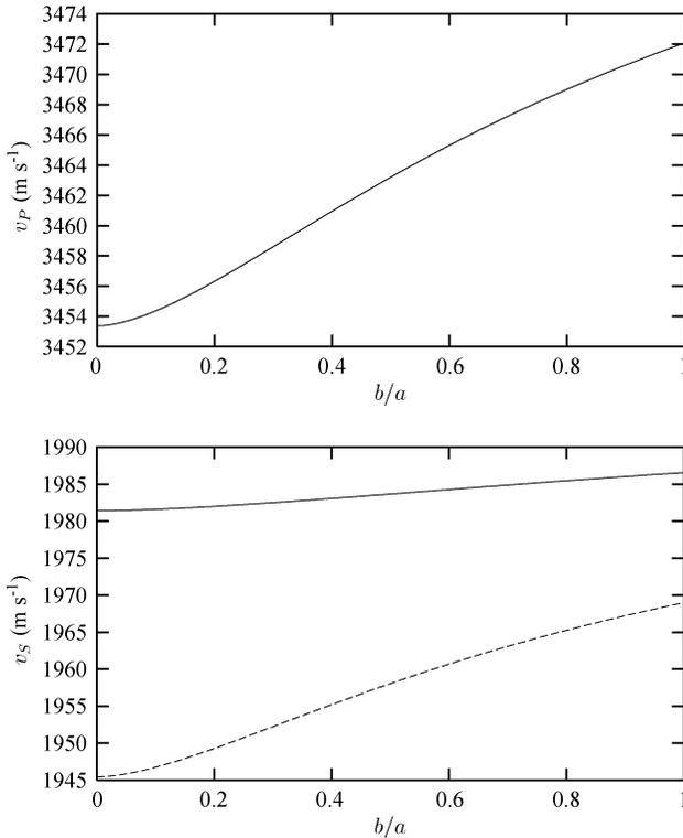
**Figure 3.** (a) The variation in compressional wave speed with the ratio of the crack height to length for a fixed porosity at an offset of 30° and an azimuth of 30°. (b) As in (a), but for shear wave speeds. The solid line corresponds to the quasi-SV wave and the dashed line to the quasi-SH wave.
