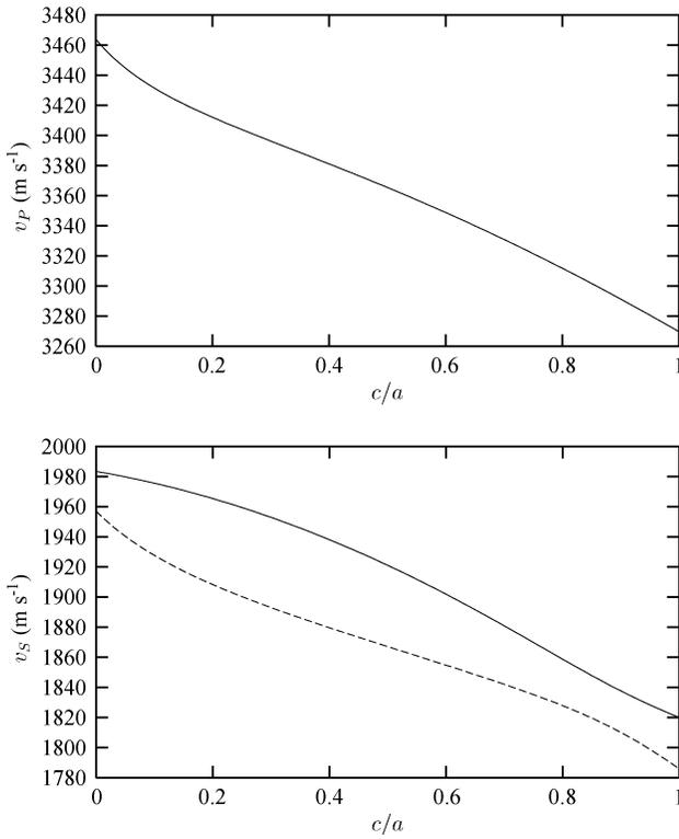
**Figure 2.** (a) The variation in compressional wave speed with the ratio of the crack width to length for a fixed crack density at an offset of 30° and an azimuth of 30°. (b) As in (a), but for shear wavespeeds. The solid line corresponds to the quasi-SV wave and the dashed line to the quasi-SH wave.
