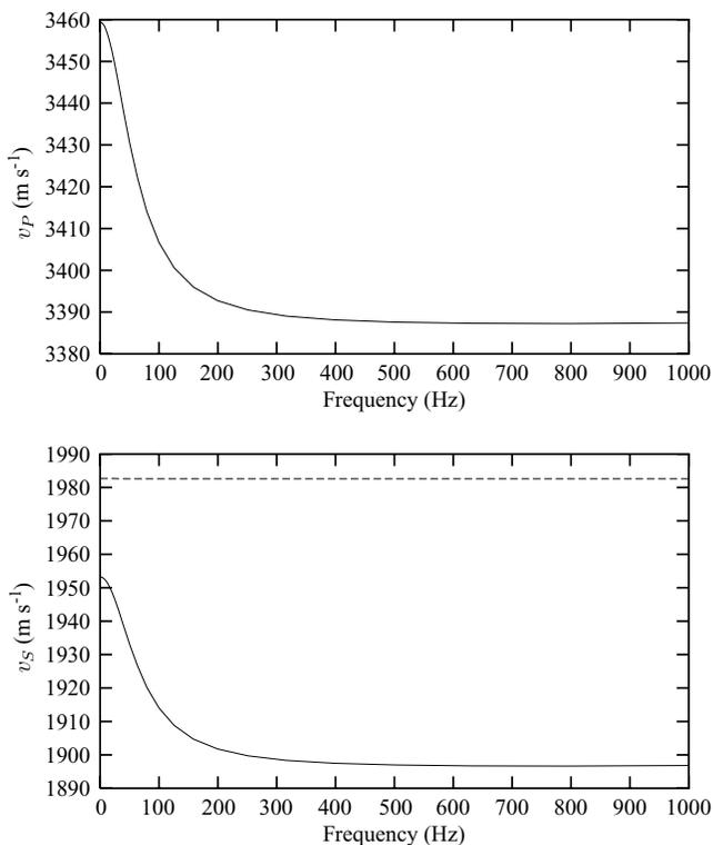
**Figure 5.** (a) As Fig. 4(a), but with  $\tau = 10^{-6}$  s. (b) As in (a), but for shear wave speeds. The solid line corresponds to the quasi-SV wave and the dashed line to the quasi-SH wave.
