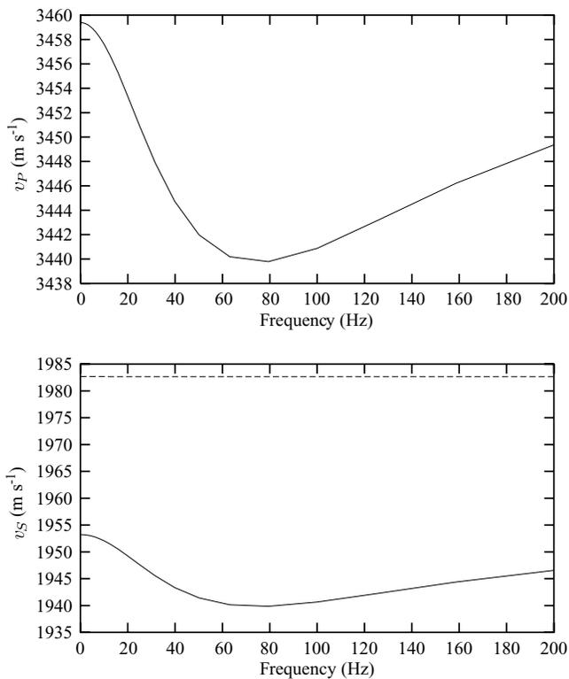
**Figure 4.** (a) The variation in compressional wave speed with frequency at  $\tau = 10^{-4}$  s and  $K'/\eta = 10^{-7}$  m<sup>2</sup> Pa<sup>-1</sup> s<sup>-1</sup>. (b) As in (a), but for shear wave speeds. The solid line corresponds to the quasi-SV wave and the dashed line to the quasi-SH wave.
