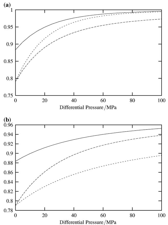
**Figure 4.** (a) Normalized compressional (solid line) and vertically and horizontally polarized shear wave speeds (long dashes, short dashes) as a function of differential pressure, at a fluid pressure of 0 MPa, at incidence normal to the direction of symmetry, under biaxial compression. (b) As in (a), except under uniaxial compression.
