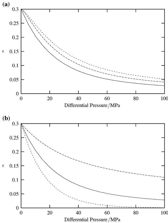
**Figure 1.** (a) Crack density  $\epsilon$  as a function of differential pressure at 0 MPa (solid line), 10 MPa (long dashes) and 20 MPa (short dashes) fluid pressure, under biaxial compression. (b) Crack density as a function of differential pressure for fluid pressure 0 MPa under biaxial (solid line), uniaxial (long dashes) and hydrostatic (short dashes) compression.
