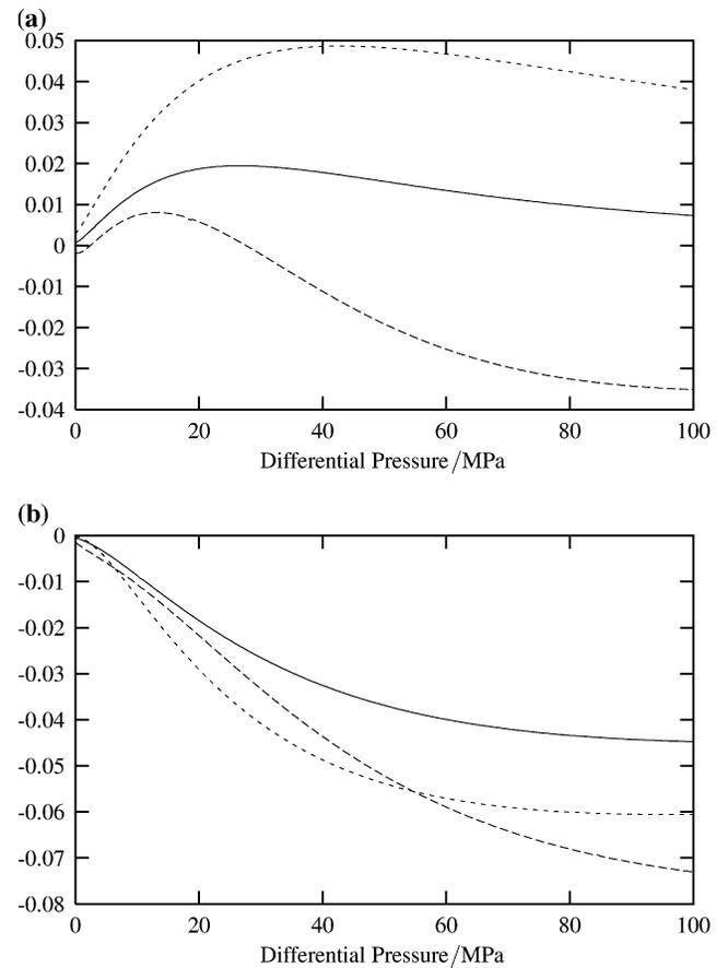
**Figure 2.** (a) Thomsen's parameters  $\epsilon_T$  (solid line),  $\delta_T$  (long dashes) and  $\gamma_T$  (short dashes) as a function of differential pressure at a fluid pressure of 20 MPa, under biaxial compression. (b) As in (a), except under uniaxial compression.
