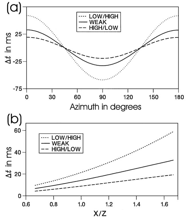
FIG. 1. Variations of AMR for the three models from Table 1. (a) Variations with azimuth at constant offset  $x = 3000$  m; (b) variations with offset-depth ratio ( $x/z$ ) of the moveout difference calculated between the two azimuths parallel ( $0^\circ$ ) and perpendicular ( $90^\circ$ ) to the fracture strike.
