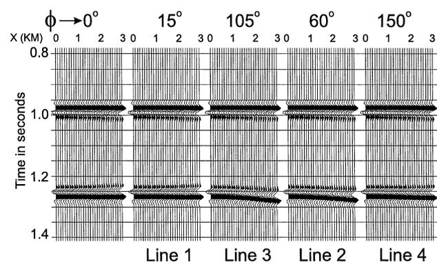
FIG. 3. CDP gathers for five different azimuths calculated for the shale/fractured gas sand model (model 3 in Table 1) with a high/low impedance contrast.
