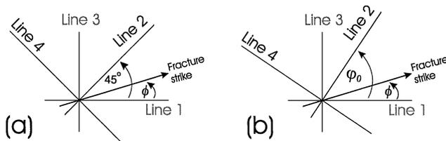
FIG. 2. Four-line configuration: (a) 45° separation; (b) separation by angle  $\phi_0$ . Lines 1 and 3 form a right-handed coordinate system, with the third axis pointing to the reader. The value  $\phi$  is the angle between line 1 and the fracture strike; positive  $\phi$  indicates a counterclockwise rotation, while negative  $\phi$  indicates a clockwise rotation.
