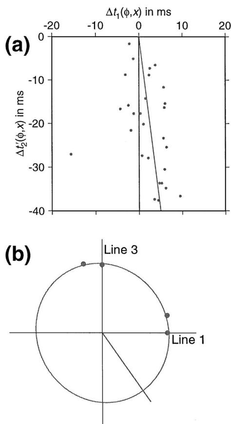
FIG. 7. (a) Crossplot of  $\Delta t_1(x)$  versus  $\Delta t'_2(x)$  obtained from Figure 6. (b) The interval NMO ellipse built from Table 3. The long axis is 3782 m/s, and the short axis is 3516 m/s with about 10% change.
