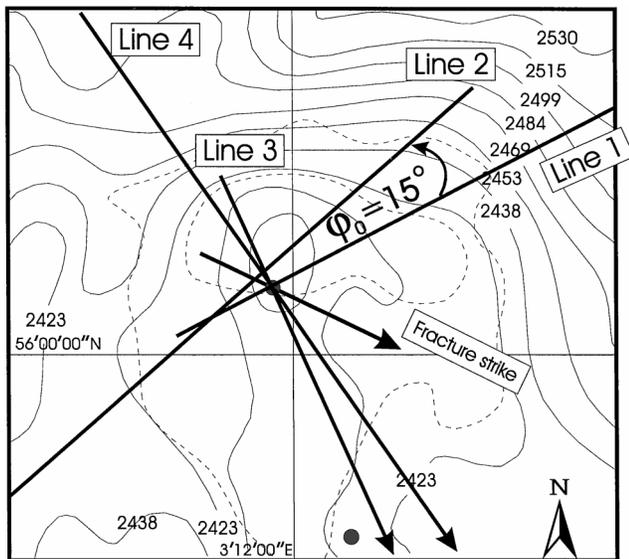
FIG. 5. Field data example. Map of the four seismic lines from the North Sea. Lines 1 and 3 intersect each other at CDPs 420 (line 1) and 440 (line 3), while lines 2 and 4 intersect at 730 (line 2) and 830 (line 4).
