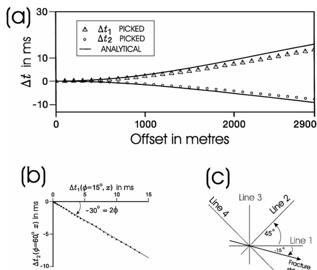
FIG. 4. (a) Comparison of the moveouts picked from Figure 3 with those calculated using equation (13) for model 3 in Table 1. (b) The crossplot of  $\Delta t_1(15^\circ, x)$  versus  $\Delta t_2(60^\circ, x)$ . (c) The relationship between the fracture strike and the survey lines.
