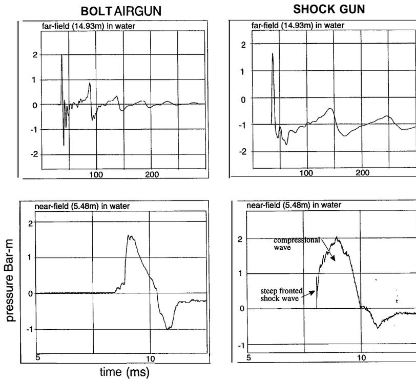
**Figure 1.** Tests at Wraysbury reservoir. Near- (5.48 m) and far-field (14.83 m) signatures are recorded from a Bolt airgun with a chamber volume of 20 in<sup>3</sup> and the shock gun with its 300 in<sup>3</sup> chamber filled with helium. Both guns were fired at 1500 psi into the omnidirectional ball hydrophones which are positioned directly below the source. The air-gun signatures are sampled at 50 000 samples/s and the shock gun at 100 000 samples/s.
