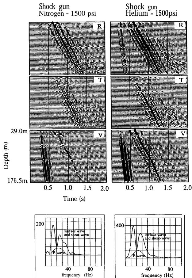
**Figure 4. Rotated 3-C data recorded at a depth of 176.5 m in a VSP configuration at the Shell test site. The shock gun is operated on land at an offset of 23 m, with two different gases at 1500 psi. The lower part of the diagram shows the resultant amplitude spectra.**
