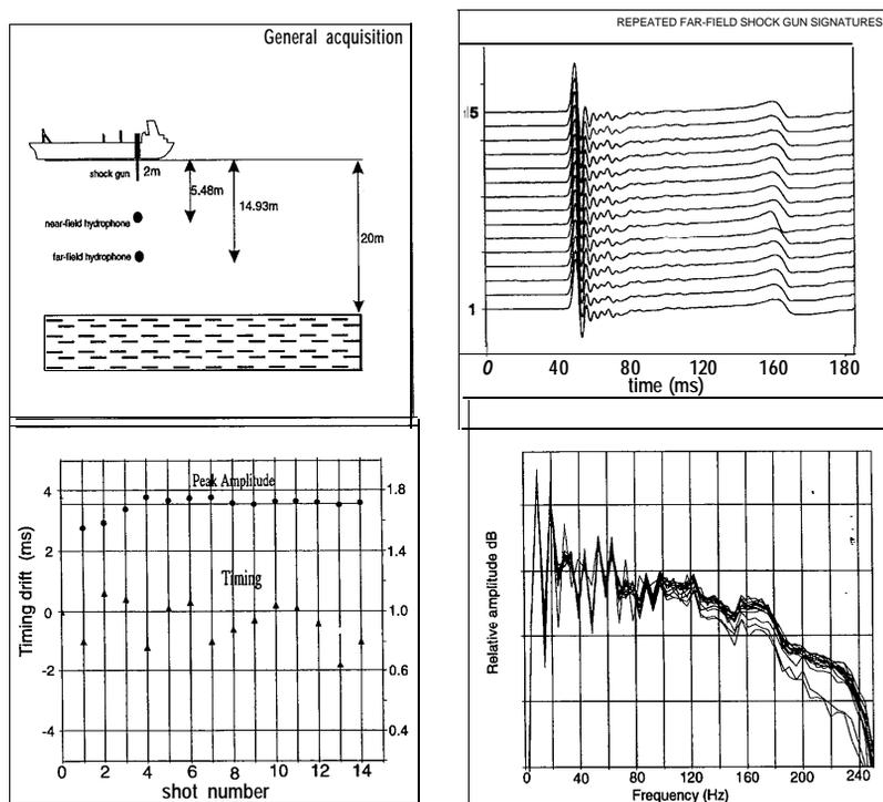
**Figure 2.** Repeated far-field signatures for the shock gun at 1500 psi in the Wraysbury tests, together with time breaks, amplitudes, and spectra. The signatures are sampled every 1/20 ms. The standard deviation for the timing is 0.70 ms, and 0.058 bar-m for the amplitudes.
