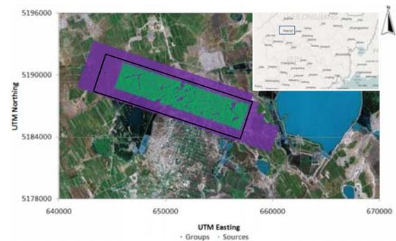
Figure 2. The geometry of 3D acquisition in the Daqing oilfield. The green markers show locations of dynamite sources and purple points indicate receiver locations.
