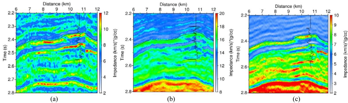
**Figure 6.** Inverted section of RI (150ms/km), EI (48°) and  $\tilde{R}I$  (150ms/km) for the reservoir in case 2. Gas-sand is represented by high impedance value. Corresponding well logs are plotted.
