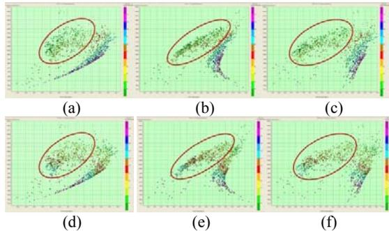
**Figure 5.** (a) – (c) Cross-plots of AI with RI (150ms/km), EI (42°) and  $\tilde{R}I$  for case 3, colour key represents gamma ray and porosity. Same as (a) – (c), colour key represents porosity. Sands are marked with red circles.
