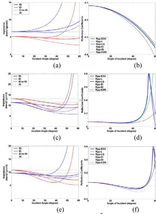
**Figure 1.** Comparison of RI, EI and  $\tilde{R}I$  for the three models in Table 1: (a) Model 1, (c) Model 2 and (e) Model 3. AVO curves for the three models are shown in (b), (d) and (f).
