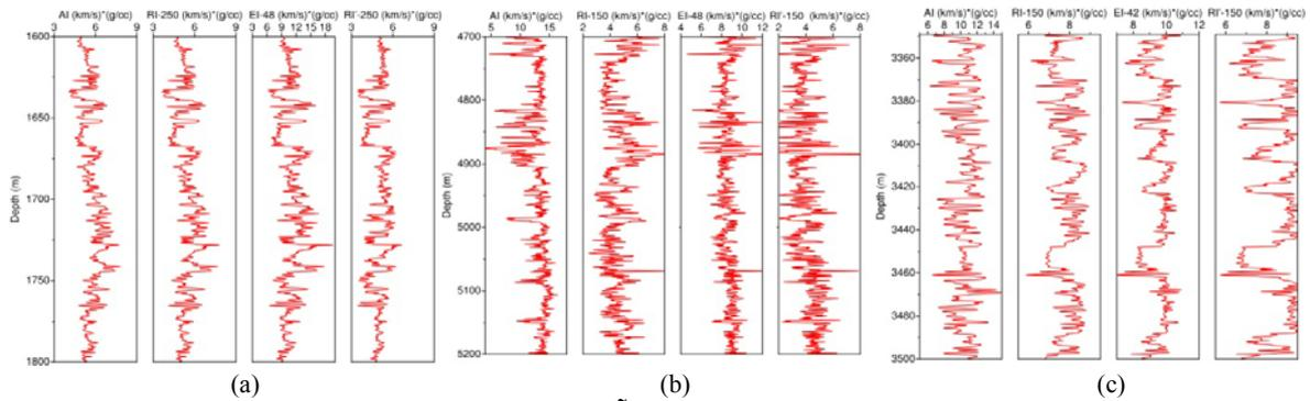
**Figure 2.** Comparison of AI with RI, EI and  $\hat{R}I$  for the wells in (a) case 1, (b) case 2 and (c) case 3.
