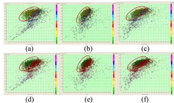
**Figure 4.** (a) - (c) Cross-plots of AI with RI (150ms/km), EI (45°) and  $\hat{R}I$  (150ms/km) for case 2, colour key represents gamma ray. (d) – (f) Same as (a) – (c), colour key represents porosity. Sands are marked with red circles.
