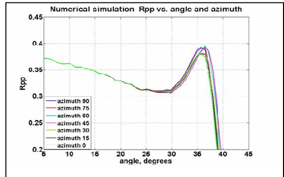
Figure 5. Numerical simulation Rpp amplitudes for water/HTI interface, plotted against incident angles of incidence and azimuths.
