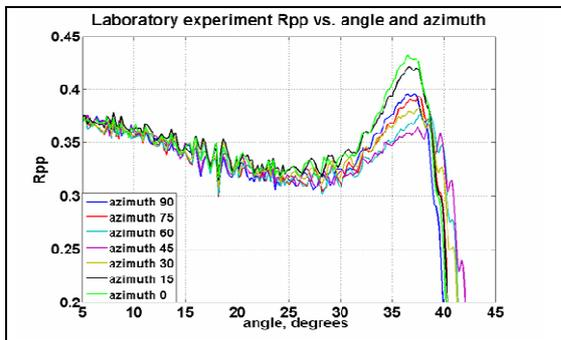
Figure 3. Laboratory experiment Rpp amplitudes for water/HTI interface, plotted against angle and azimuths.
