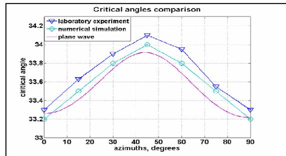
Figure 6. Comparison between critical angles computed from laboratory experiment, numerical simulations, and Snell's law at different azimuths.
