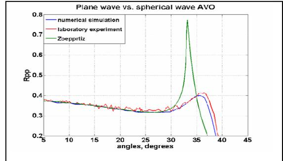
Figure 4. Rpp reflection amplitudes with applied geometrical spreading for water/isotropic model interface are plotted against angle of incidents using Zoeppritz equation (green curve). Laboratory and numerical simulation AVO responses are also shown (red and blue curves respectively).
