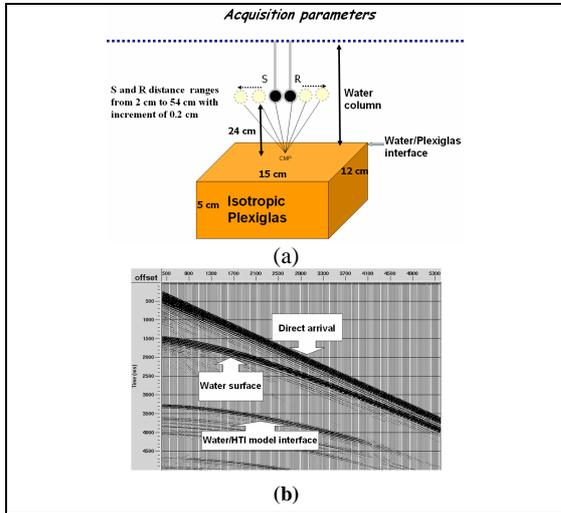
Figure 1. (a) Acquisition parameters used to perform reflection measurement out of water/ isotropic Plexiglas interface producing CMP gathers (b) with three seismic events indicated by arrows.
