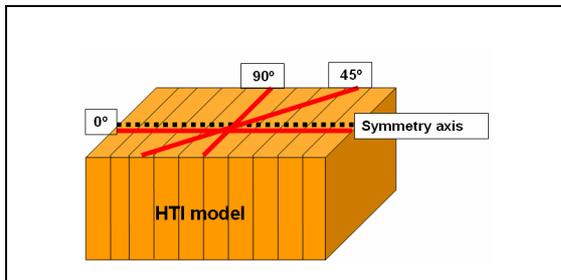
Figure 2. Azimuthal recordings at 0°, 45° and 90°. The black dotted line is the symmetry axis and the red one is the 2D CMP line azimuth direction.
