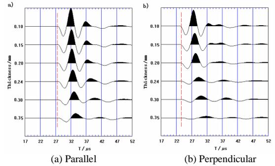
Figure 3. Comparison of P-waves recorded for the fracture models with different thickness, propagating (a) parallel and (b) perpendicular to the fractures.
