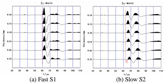
Fig. 5. Comparison of (a) the fast S1 and the slow S2 waves recorded for the fracture models with different thickness, propagating parallel to the fractures along the X-axis.
