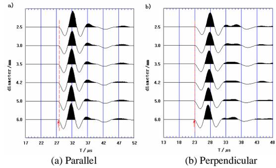
Figure 2. Comparison of P-waves recorded for the fracture models with different diameter, propagating (a) parallel and (b) perpendicular to the fractures.
