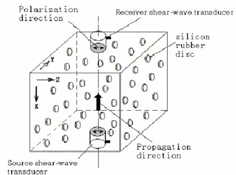
Figure 1. The controlled fracture model using epoxy resin and round chips of silicon rubber.
