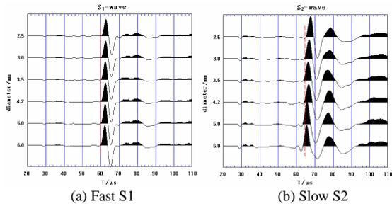
Figure 4. Comparison of (a) the fast S1 and the slow S2 waves recorded for the fracture models with different diameter, propagating parallel to the fractures along the X-axis.
