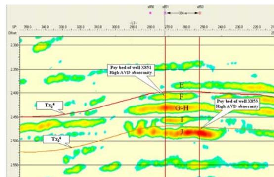
Figure 9: Absorption and velocity dispersion calculated from the P- and S-wave data for Line L3.
