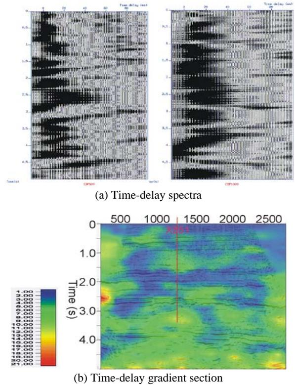
Figure 6. Shear-wave splitting analysis: (a) Calculated time-delay spectra of the split shear-waves for Line L3, and (b) interpretation results of the time-delay gradient section superimposed by the corresponding seismic section. X851 is the most productive gas well in the study area, which is drilled into a zone with more than 12 % shear-wave anisotropy. The color bar on the left indicates percentage shear-wave splitting.
