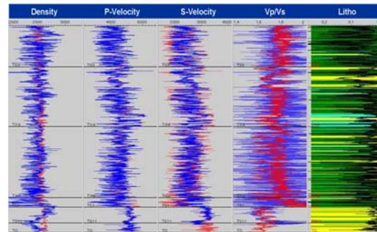
Figure 8: Sonic logs and lithology from borehole X851. Yellow color at the lithology log at the far right stands for gas sand, green for shale, and light blue for calcite.
