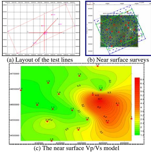
Figure 2: The acquisition programme: (a) Acquisition layout of the test lines, and the red box indicates the 3D coverage, (b) locations of micro-refraction surveys marked by the blue points and multicomponent uphole marked by the red points, and (c) the near surface Vp/Vs model derived from the surveys in (b).
