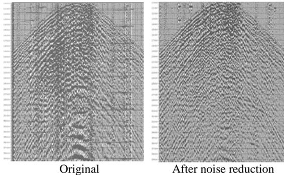
Figure 4. Comparison of the results of noise reduction, and the input data is a shot record of the inline X-component from Line 3. (a) Original data and (b) results after applying a model-based technique (Qian and Zhao, 2003).
