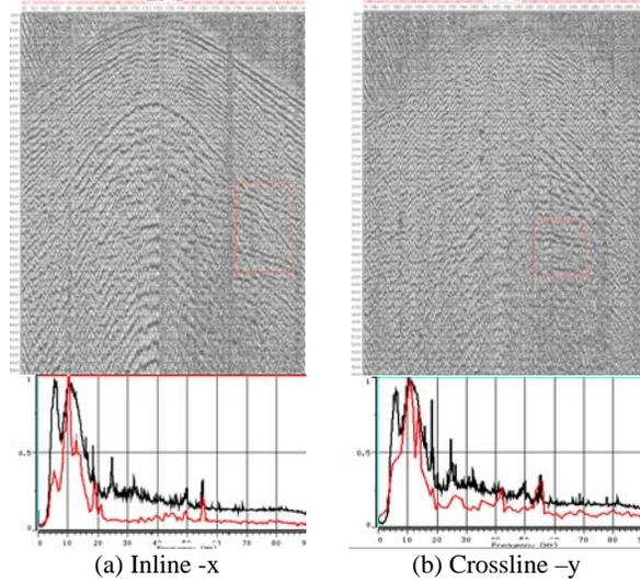
Figure 3. Sample shot records from Line 3 and their corresponding frequency spectra: (a) inline and (b) crossline horizontal components. The black curves in the spectra are calculated from the whole trace, and the red curves are calculated from the selected windows indicated by the red rectangles in the shot records.
