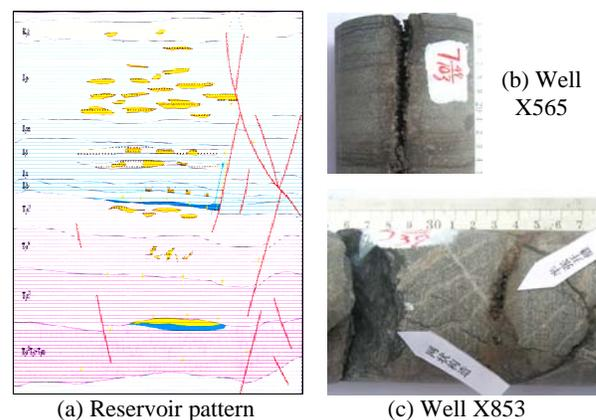
Figure 1: (a) A typical geological section showing the gas reservoir patterns, and (b) and (c) core samples from the study area.
