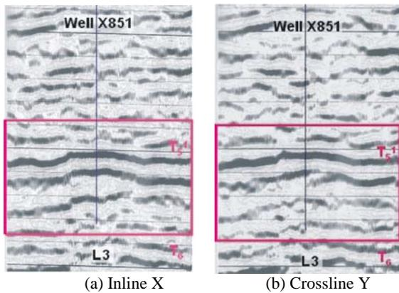
Figure 5. Final stacked sections of the horizontal (a) X- and (b) Y-components of Line L3. The red boxes highlight the target.
