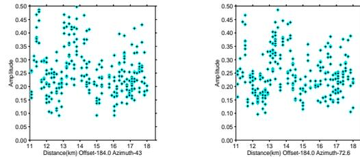
**Figure 10.** Amplitude variations with CDP points at a given offset for azimuths at 43 (left) and 73 (right) degrees.
