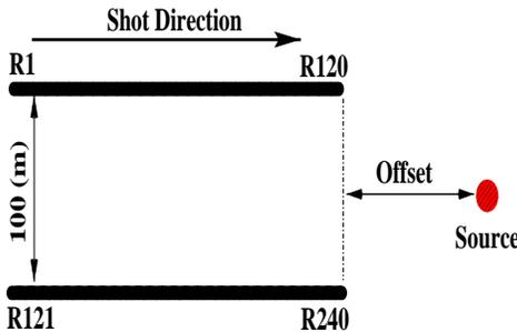
Figure 2. Streamer configuration of the 3D survey. It was a two-streamer 3D boat with 240 receivers on each streamer.
