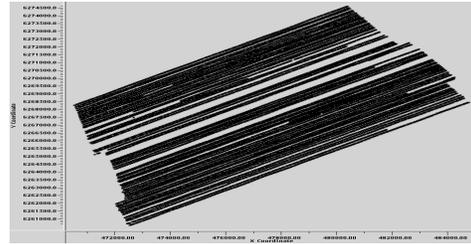
Figure 3. Regional coverage of the 3D survey. There are 88 swathes separated by 100m from each other.
