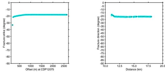
**Figure 11.** Results of azimuth AVO analysis. The fracture orientation calculated for each offset distribution for a given CDP (left) and the fracture orientation for each CDP along a given crossed 2D line (right).
