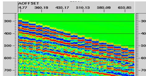
Figure 4. A windowed display of a super gather of the combined 2D and 3D surveys. Common-offset traces with different azimuths show constant first break times, and the attribute analysis will be performed on these common-offset traces.
