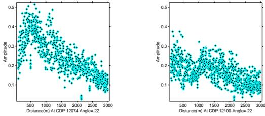
**Figure 8.** Variations of amplitude with offset for a given azimuth. Left - CDP 12074; right - CDP 12100.
