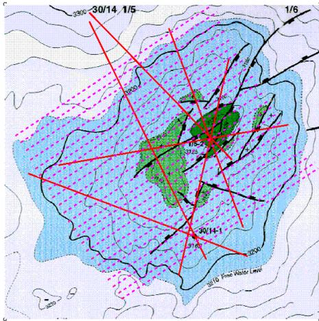
Figure 1. Depth map of the target (Ekofisk). The dashed lines show the shot direction of the 3D swathes, and the solid lines show the crossed 2D lines. There are total 88 swathes which are parallel to each other and ten 2D lines across the 3D area.
