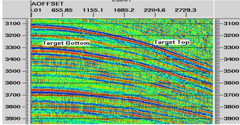
**Figure 7.** The top and bottom reflections from the target as identified in the super gather of the combined 2D and 3D surveys.
