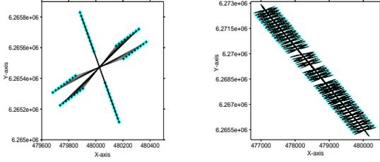
**Figure 6.** Azimuth distribution analysis. Left - the distribution for a given CDP. Right - the distribution for all CDPs along a crossed 2D line
