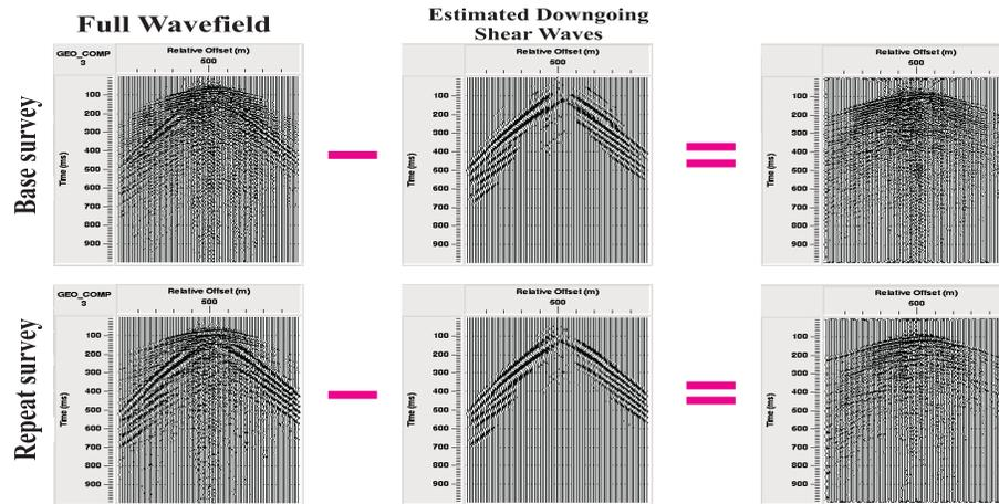
Figure 5: An example of up- and downgoing wavefield separation based on the filtering in  $t - f$  domain.
