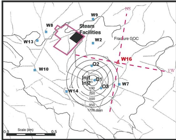
Figure 2: Expected design scenario for the steam pilot and schematic view on the walkaway VSP acquisition.
