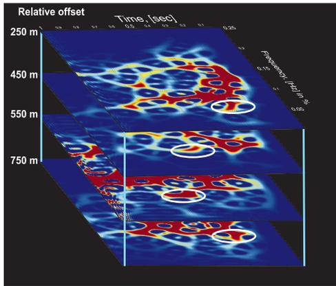
Figure 3: Filtering in  $t - f$  domain. White circles indicate selected wave mode(downgoing shear waves) to be suppressed.
