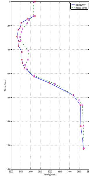
Figure 4: Velocity model for base and repeat surveys.
