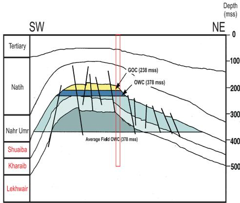
Figure 1: Cross-section of the field which contains an Aptian Shuaiba - Kharab - Lekhwair carbonate reservoir. The position of the well and the current fracture fluid contact and oil-water contact levels are indicated.
