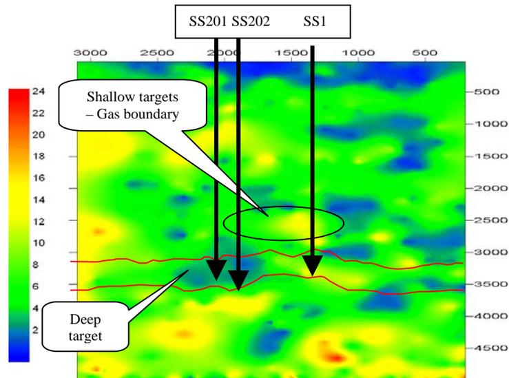
**Figure 5:** Interpretation results on the time-delay gradient section. SS202 and SS1 are gas-producing wells, and SS201 is a dry hole.
